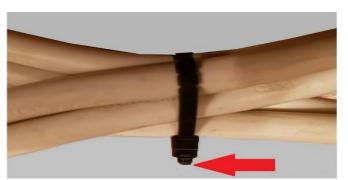
No sharp edge after tail is removed
